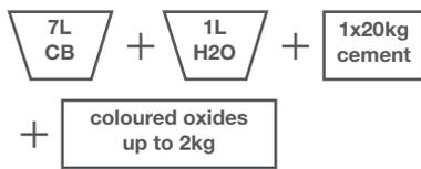
Concrete Bond 7 litres and clean water 1 litre. Add to 1 x 20kg bag of cement until desired consistency is achieved. This mix may be applied by trowel, spatula, brush, roller or through a hopper gun. Colour oxides may be used as required.
